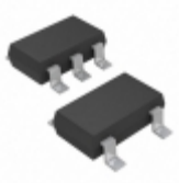
MIC5319-1.85BD5 Microchip Technology IC REG LDO 1.85V 0.5A TSOT23-5
