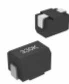
CM453232-3R3JL Bourns Inc. FIXED IND 3.3UH 355MA 800 MOHM
