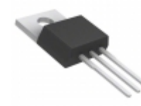
BDX34BTSTU AMI Semiconductor / ON Semiconductor TRANS PNP 80V 10A TO-220
