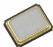
FA-128 27.1200MA10V-C0 EPSON CRYSTAL 27.1200 MHZ 18.0PF SMD
