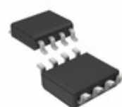
LE50CD-TR STMicroelectronics IC REG LDO 5V 0.1A 8SO
