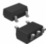
S-1000C41-M5T1U SII Semiconductor Corporation IC VOLT DETECTOR
