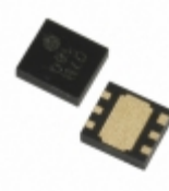
XC6121D734ER-G Torex Semiconductor Ltd IC WATCHDOG TIMER 6-USP
