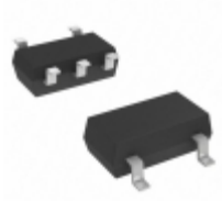
MIC5253-3.0YC5-TR Microchip Technology IC REG LDO 3V 0.1A SC70-5
