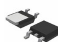
MC79M12BDTG ON Semiconductor IC REG LDO -12V 0.5A DPAK
