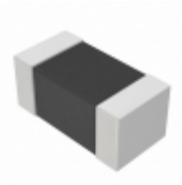
LQM18PN4R7MFRL Murata Electronics North America FIXED IND 4.7UH 620MA 550 MOHM
