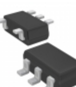
XC6123E618MR-G Torex Semiconductor Ltd IC WATCHDOG TIMER SOT-25
