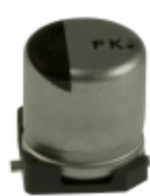
EEE-FK1C220AR Panasonic Electronic Components CAP ALUM 22UF 20% 16V SMD
