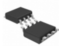
LTC1798CS8-4.1#PBF ADI (Analog Devices, Inc.) IC VREF SERIES 4.096V 8SOIC
