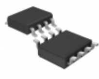
LTC1798CS8-2.5#TRPBF Linear Technology IC VREF SERIES 2.5V 8SOIC
