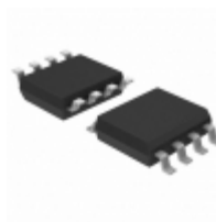
EL5160IS-T13 Intersil IC OPAMP CFA 200MHZ 8SOIC
