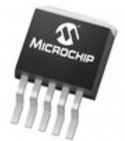
MCP1826-2502E/ET Microchip Technology IC REG LDO 2.5V 1A DDPAK
