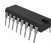
DM74LS85N Fairchild/ON Semiconductor IC COMPARATOR MAGNITUDE 4B 16DIP
