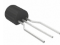
KSP2222ATA Fairchild/ON Semiconductor TRANS NPN 40V 0.6A TO-92
