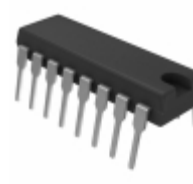
AD7249BN Analog Devices Inc. IC DAC 12BIT SRL W/REF 16-DIP
