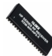
RXM-900-HP3-SPS LinX Technologies Inc. RECEIVER RF 902-928MHZ 8P/100S
