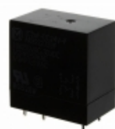
JC2AF-DC24V Panasonic Electric Works RELAY GEN PURPOSE DPST 10A 24V
