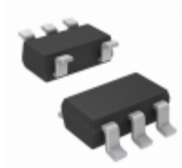
MCP73831T-2ACI/OT Microchip Technology IC CONTRLLR LI-ION 4.2V SOT23-5
