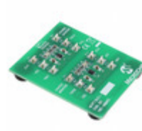
MCP73831EV Micrel / Microchip Technology BOARD DEMO FOR MCP73831
