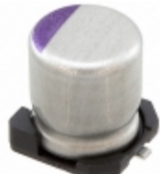
16SVPS39M Panasonic Electronic Components CAP ALUM POLY 39UF 20% 16V SMD
