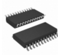
AD7890BR-4 Analog Devices Inc. IC DAS 12BIT 8CH 24-SOIC
