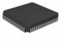
PIC18LF6585-I/L Microchip Technology IC MCU 8BIT 48KB FLASH 68PLCC
