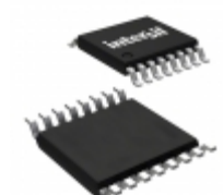
HIN202EIBZ-T Intersil IC 2DRVR/2RCVR RS232 5V 16- SOIC
