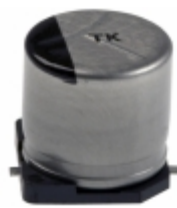
EEE-TKA332UAM Panasonic Electronic Components CAP ALUM 3300UF 20% 10V SMD
