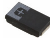
6TPE100M Panasonic Electronic Components CAP TANT POLY 100UF 6.3V 2917
