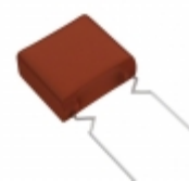
ECW-F2335HAQ Panasonic Electronic Components CAP FILM 3.3UF 3% 250VDC RADIAL
