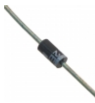
1N4732PE3/TR12 Microsemi Corporation DIODE ZENER 4.7V 1W DO204AL
