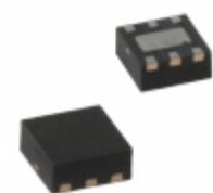
MIC5321-PJYMT-TR Microchip Technology IC REG LDO 3V/2.5V 0.15A 6TMLF
