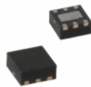
MIC5321-PPYML-TR Microchip Technology IC REG LDO 3V 0.15A 6MLF
