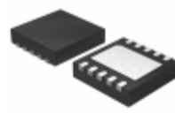
LTC3536IDD#TRPBF ADI (Analog Devices, Inc.) IC REG BCK BST ADJ 1A SYNC 10DFN
