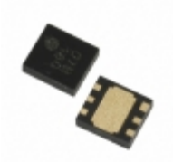
XC6122F633ER-G Torex Semiconductor Ltd IC WATCHDOG TIMER 6-USP
