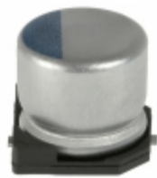
APXH4R0ARA151MF60G United Chemi-Con CAP ALUM POLY 150UF 20% 4V SMD
