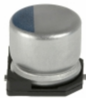
APXH160ARA390MF60G United Chemi-Con CAP ALUM POLY 39UF 20% 16V SMD
