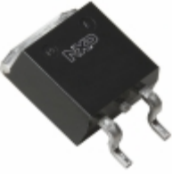
BUK9640-100A,118 Nexperia USA Inc. MOSFET N-CH 100V 39A D2PAK
