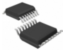
LTC2619IGN#TRPBF Linear Technology IC DAC 14BIT R-R QUAD 16SSOP
