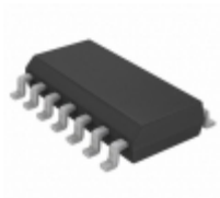
MCP42010T-I/SL Microchip Technology IC POT DGTL 10K 2CH SPI 14-SOIC
