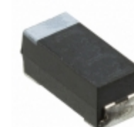
CWR29KC226JCGC AVX Corporation CAP TANT 22UF 5% 25V 2711
