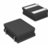
LQH2HPN4R7MJRL Murata Electronics North America FIXED IND 4.7UH 770MA 204 MOHM
