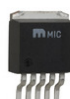
MIC39151-1.65WU Microchip Technology IC REG LDO 1.65V 1.5A TO263-5
