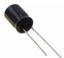
EEU-FC0J471BJ Panasonic Electronic Components CAP ALUM 470UF 20% 6.3V RADIAL
