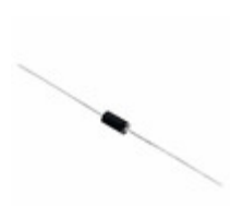
P6KE27CA Littelfuse Inc. TVS DIODE 23.1VWM 37.5VC DO204AC
