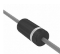
P6KE27CA-E3/54 Vishay Semiconductor Diodes Division TVS DIODE 23.1VWM 37.5VC DO204AC
