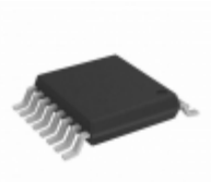
MC68HC908QY1CDT NXP USA Inc. IC MCU 8BIT 1.5KB FLASH 16TSSOP
