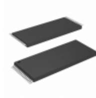
AT49F040A-70TU Microchip Technology IC FLASH 4MBIT 70NS 32TSOP
