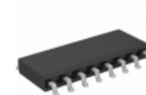
MC74ACT138DR2G ON Semiconductor IC DECODER/DEMUX 1-8 HS 16SOIC
