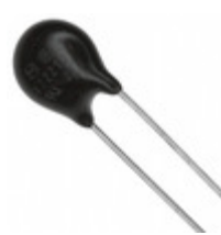
ERZ-V07D680 Panasonic Electronic Components VARISTOR 68V 500A DISC 7MM
