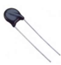
ERZ-V10D101 Panasonic Electronic Components VARISTOR 100V 3.5KA DISC 10MM
