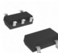
S-80147ANMC-JC8T2G SII Semiconductor Corporation IC VOLT DETECTOR 4.7V SOT23-5
