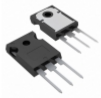
STGW40V60DLF STMicroelectronics IGBT 600V 80A 283W TO247
