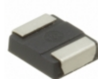
10TPG47M Panasonic Electronic Components CAP TANT POLY 47UF 10V 1411
