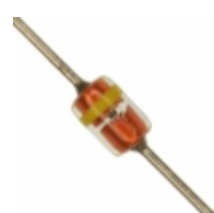
MTZJT-7718B Rohm Semiconductor DIODE ZENER 18V 500MW MSD
