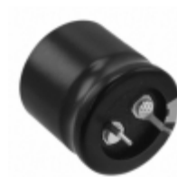
ECO-S1VP472CA Panasonic Electronic Components CAP ALUM 4700UF 20% 35V SNAP
